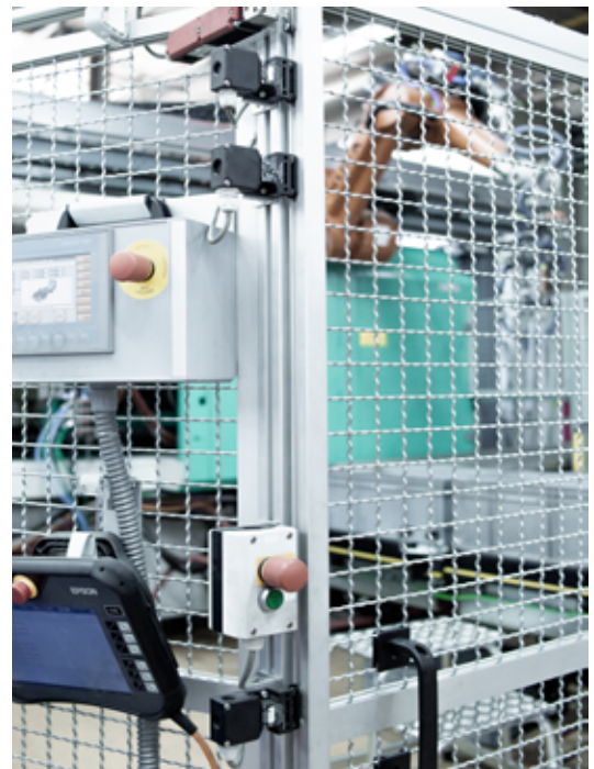
EUROMAP 73 protection with three safety switches on the safety door.
