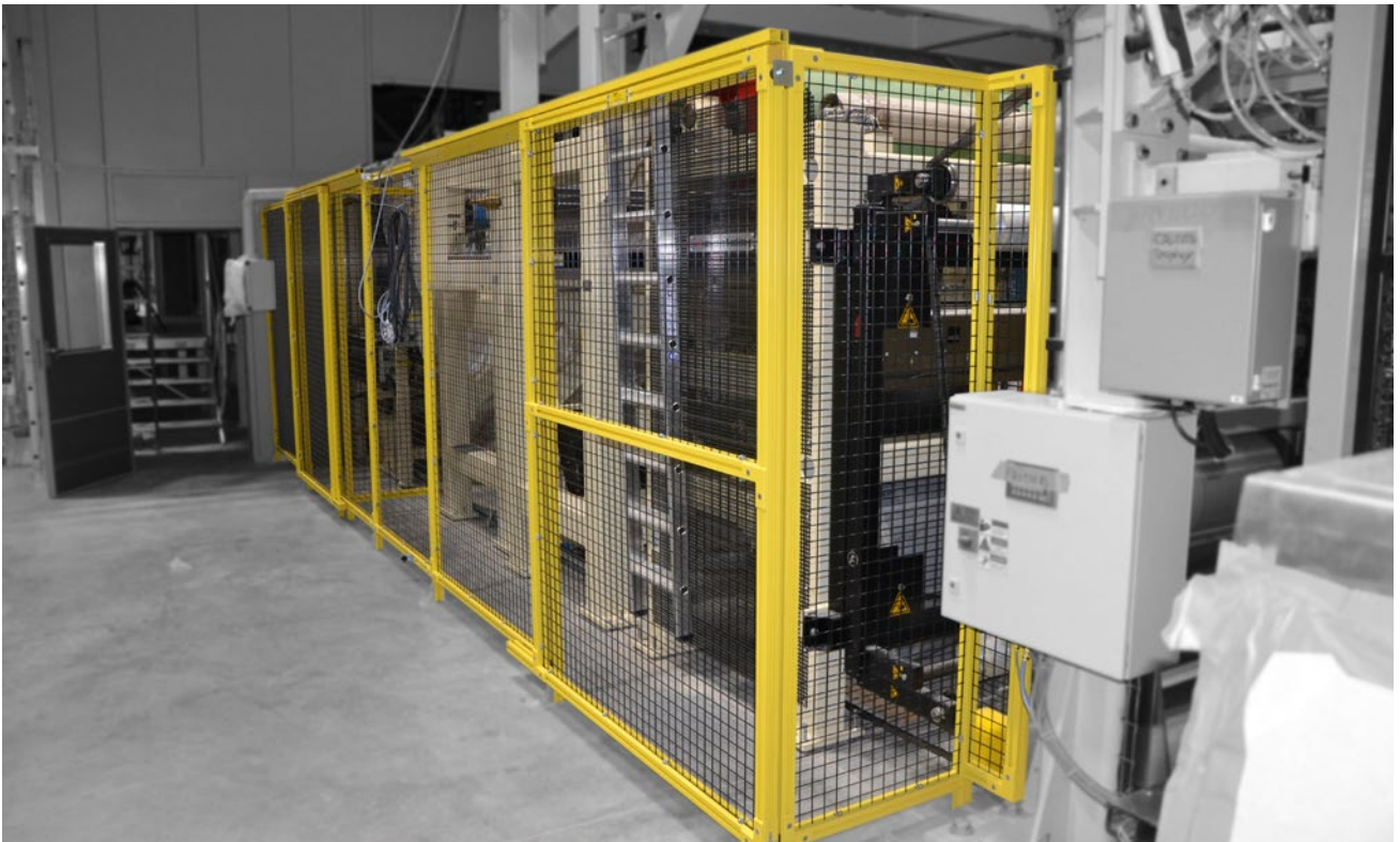
Sliding gate with yellow powdered aluminum profile
