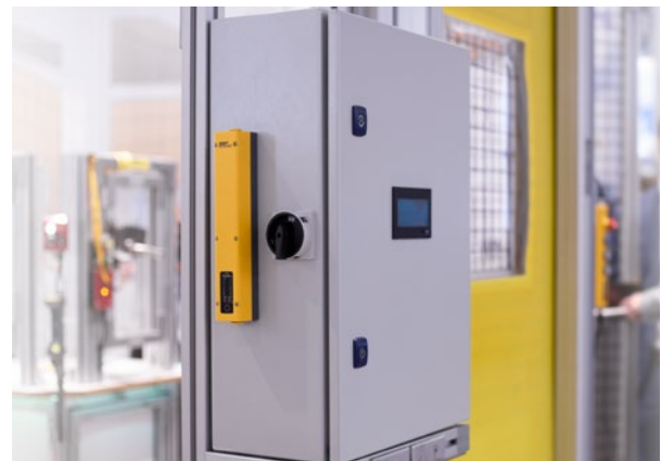
The gate control can be combined with the Safety Simplifier safety controller
