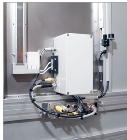
I/O link or Profinet connection
